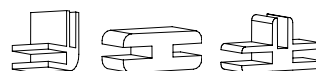
2-Way & 3-Way Connector Clips Corner, T, and Straight Connectors for Clear and Frosted Acrylic Options (See Details)
