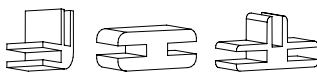
2-Way & 3-Way Connector Clips Corner, T, and Straight Connectors for Clear and Frosted Acrylic Options
