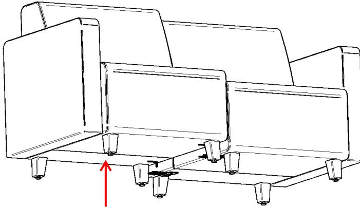
*Note: You will only need to lift the unit approx. 2" to remove the L bracket from the 2-prong portion of the ganging bracket.*
