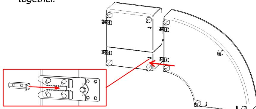
8 The two units should be fully ganged and should not pull apart.
