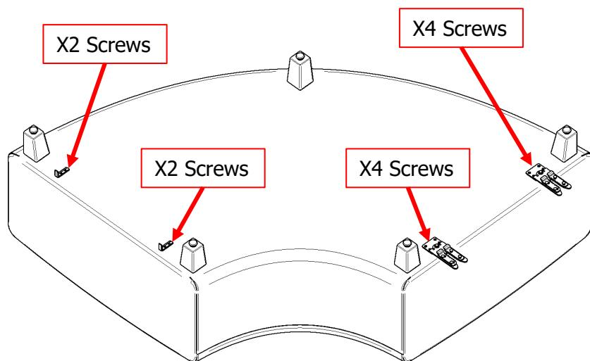
5 Use the paper template #1 for the prong side of the ganging bracket. Fold the template on the fold line. Align the edge of the template flush with the front edge of the seat. Position bracket into the corner of the template & reinstall the screws. Repeat for the other side.
