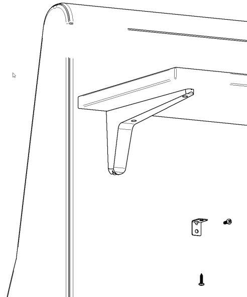
**6** Without applying too much torque, attach the "L" brackets to the underside of the table and to the back of the unit utilizing the #8 screws.
