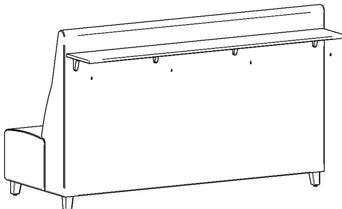
4 Pushing the table against the back of the unit so no gap is left between the table and the fabric, insert the #12 flat head screws into the brackets and into the table.
