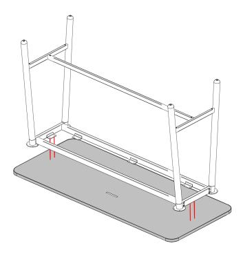
Install #10 x 7/8" screws into the 32 holes in the base assembly.
