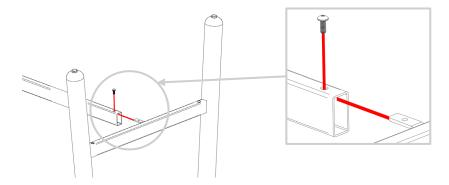
Attach the other end frame assembly using the  $\frac{1}{4}$ -20 x 2-3/8" bolts and the  $\frac{1}{4}$ -20 x  $\frac{1}{2}$ " bolt. Similar to steps 2 & 3.
