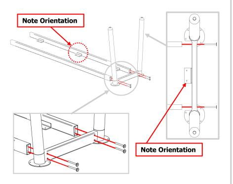
Attach the other end frame assembly using the  $\frac{1}{4}$ -20 x 2-3/8" bolts. Similar to step 2.
