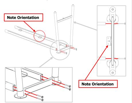
Attach the lower stretcher rail to the end frame using the  $\frac{1}{4}$ -20 x  $\frac{1}{2}$ " bolt.
