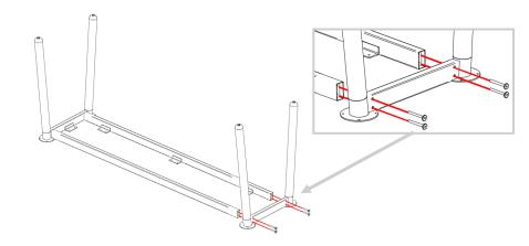
4 Double check to make sure all the bolts on the base assembly are tight.
