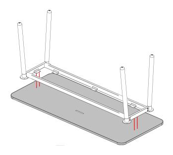
6 Install #10 x 7/8" screws into the 32 holes in the base assembly.
