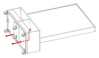
For 82-4872PMLS & 82-4872PMLOS units, wires can be run on either side of the center divider.
