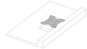
VESA Mounting Plate hole patterns 75mm x 75mm 100mm x 100mm 100mm x 200mm 200mm x 200mm
