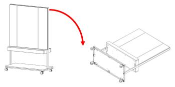
Attach the 4 casters to the bottom of the unit using the provided bolts.
