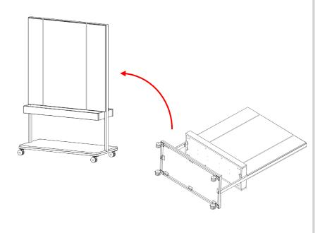
Once the unit is stood upright. The straps around the panels can be removed. Also be sure to firmly push down on both panels to make sure they are fully seated.
