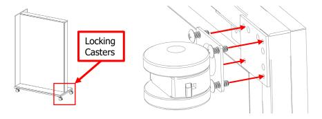
For models requiring 6 casters. Attach the 2 center non-locking casters with the provided bolts.
