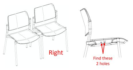
Squeeze the prongs on the female side of the 910-000GB – ganging bracket and insert into the 2 holes beneath the seat.
