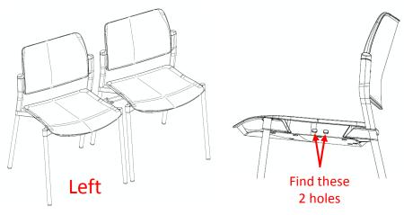
Squeeze the prongs on the male side of the 910-000GB – ganging bracket and insert into the 2 holes beneath the seat.
