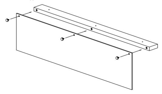
**Step 2:** Next, using the supplied *Screws*, drive the screws thru the pilot holes in the *Support Rail* up into the underneath side of the work surface. Orient the part depending upon the application. Orient *Acrylic* above the work surface for a Privacy Panel or orient *Acrylic* below the work surface for Modesty Panel
