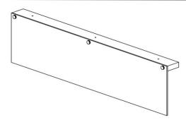
**Step 1:** Using *Stand Offs* and the supplied *Acrylic*, screw the *Stand Offs* thru the *Acrylic* and into the insert nuts mounted in the *Support rail* as shown below
