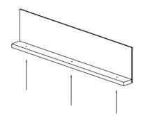
Drive Screws Up Into Work Surface
