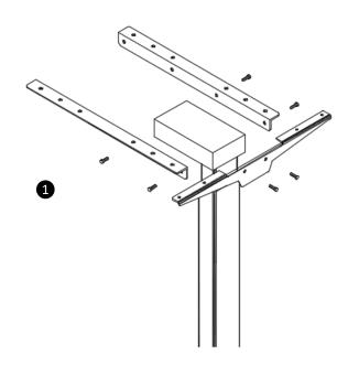
Attach worksurface by lining up L-Bracket holes with the highlighted holes shown below. Use #10 X 7/8 PPH screws provided.
