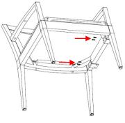
The 2 (two) 2209-00395T – L Bracket should be placed as shown.
