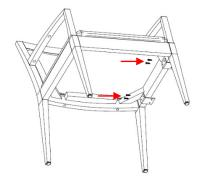
The 2 (two) 2209-00395T – L Bracket should be placed as shown.
