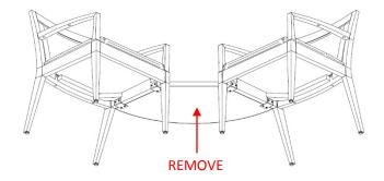
Unscrew 4 (four) 2202-01078 - #10 x 7/8 Pan Head Screw. 2 (two) screws per bracket.
