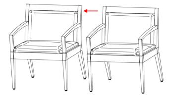
Screw brackets in place using 4 (four) 2202-01078 -#10 x 7/8 Pan Head Screw. 2 (two) screws per bracket. NOTE: Align front of legs and bottom of the seat rail before installing screws.
