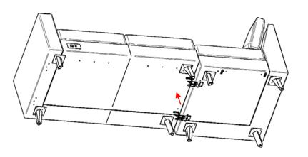
Note: You will only need to lift the seat approx. 2" to remove the L bracket from the 2-prong portion of the ganging bracket.
