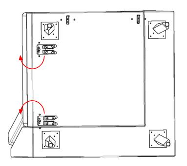
Set the second seat near the first seat so that the L-bracket on the second seat aligns with the center of the 2-prong portion on the first seat.
