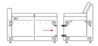
Note: The brackets will click as the seats are pushed together. Push the seats together as tight as possible.
