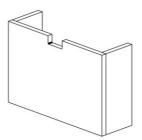
**Step 1:** Using supplied L-Brackets, fasten the U-Support to the top as shown. (Fig. A)
