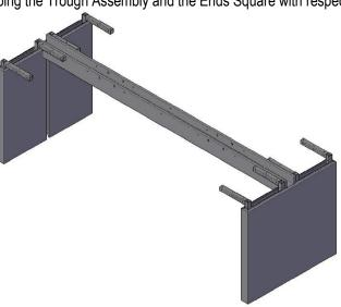
**Step 4:** Place (1) Top on the assembly and fasten to the black metal Support Brackets using the #8 x 2" Pan Head Screws **Note: the Top is placed on the inside of the trough and is flush with the ends. Be sure to push the top all the way down prior to fastening) Next, fasten the top to the trough using the pre-marked holes in the Trough and the #8 x 1-1/4" Flat head screws.**
