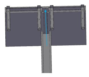
Step 3: Repeat Step 2 on the remaining End, while keeping the Trough Assembly and the Ends Square with respect to each other.
