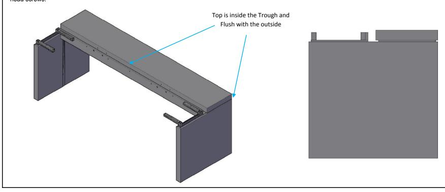
**Step 5:** Repeat **Step 4** for the remaining Top. Next *(if power modules were ordered with the table),* insert power modules and fasten per the provided instructions in the Power Module box. Now, route cords thru the acces cut out in the Ends and re-install the Metal Cord Covers from **Step 1**
