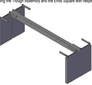
**Step 4:** Place the Top on the assembly and fasten to the black metal Support Brackets using the #8 x 2" Pan Head Screws **Note: Be sure to push the top all the way down prior to fastening)** Next, fasten the top to the trough using the supplied 2" L-Brackets and the #6 X 5/8" Pan Head Screws. Next re-install the Metal Cord Covers from **Step 1**
