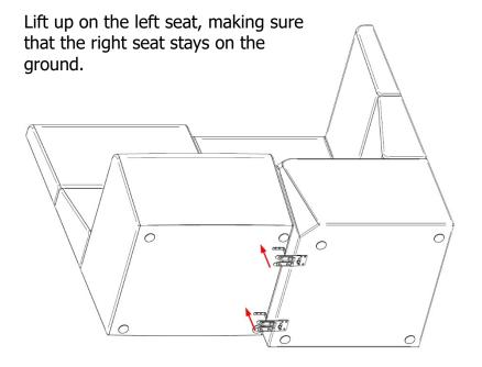
Note: You will only need to lift the seat approx. 2" to remove the L bracket from the 2-prong portion of the ganging bracket.
