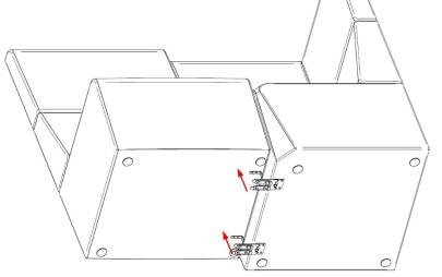
Note: You will only need to lift the seat approx. 2" to remove the L bracket from the 2-prong portion of the ganging bracket.
