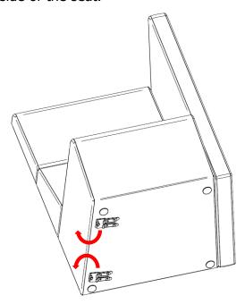
2 Set the second seat near the first seat so that the L bracket on the second seat aligns with the center of the 2 prong portion on the first seat.
