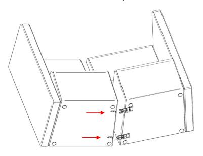
Note: The brackets will click as the seats are pushed together. Push the seats together as tight as possible.
